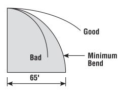
Turns in a bore path should be made gradually. The drawing illustrates the 65' bend radius. To obtain a 90° turn you will require 65' of forward distance in any directional plane.
